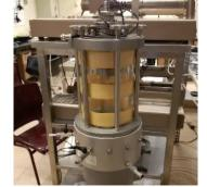
This testing system is essential for understanding how soils behave under dynamic loading conditions and is particularly valuable in earthquake engineering and geotechnical research. It allows engineers and researchers to evaluate soil response and make informed decisions regarding the design and safety of structures in earthquake-prone areas.
