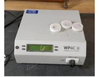
Water Potentiometer is used in geotechnics: monitoring pore water pressure, field testing, triaxial testing, slope stability analysis, foundation design, and permeability studies. Research and Data Collection: WP4 Water Potentiometers are essential for research studies in geotechnical engineering. They enable data collection related to pore water pressure and its influence on various soil behaviors, contributing to the development of more accurate models and design practices.
