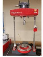
This specialized equipment is crucial in understanding how geotechnical materials respond to repeated loading conditions, which can be encountered in various construction and infrastructure projects. It provides essential data for designing safe and stable geotechnical structures and assessing the long-term performance of these structures under dynamic loads.
