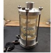
Triaxial chambers with incorporated radial deformation sensors are essential for characterizing soil properties, conducting research, and ensuring the stability and safety of geotechnical structures. Proper calibration and adherence to testing standards are crucial when using these chambers to provide accurate and reliable test results.
